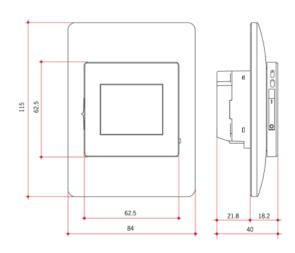
Dimensions show the 5235W complete Thermostat with the Coverplate  $\,$
