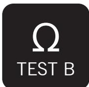
Test the resistance (using instructions on page 8) of the heating cable once installed. Compare the tested resistance to the correct resistance of the cable and ensure this is within  $-5\Omega$  to  $+ 10\Omega$ . Record the result on the customer hand over form (page 15).
