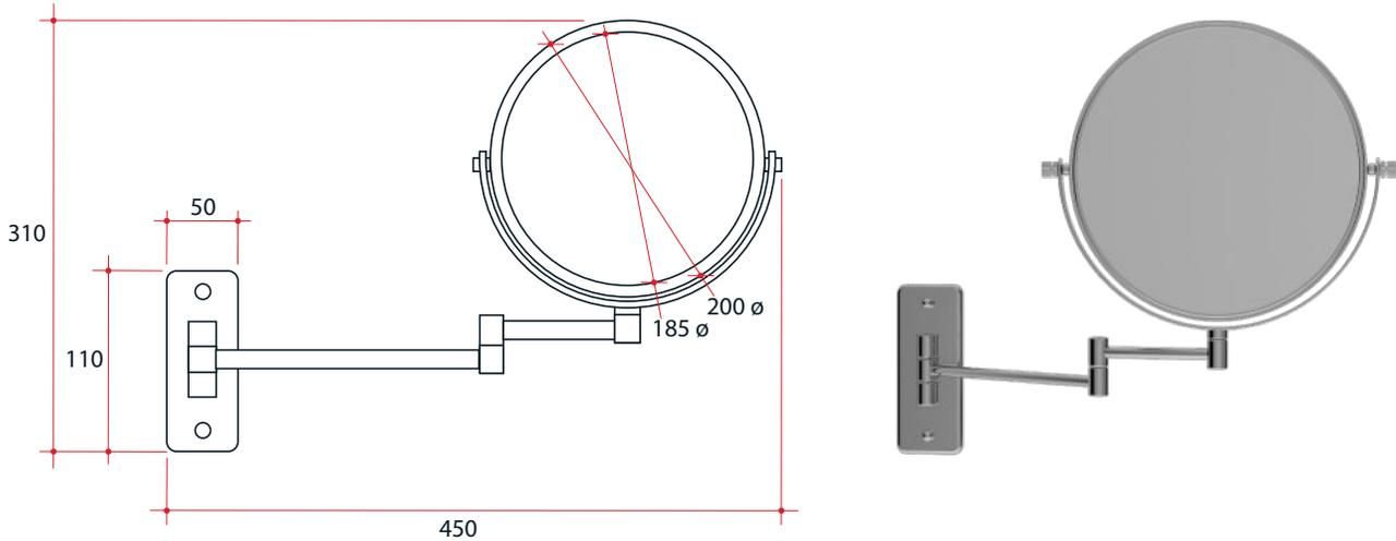
Note: All dimensions are in millimetres (mm)
