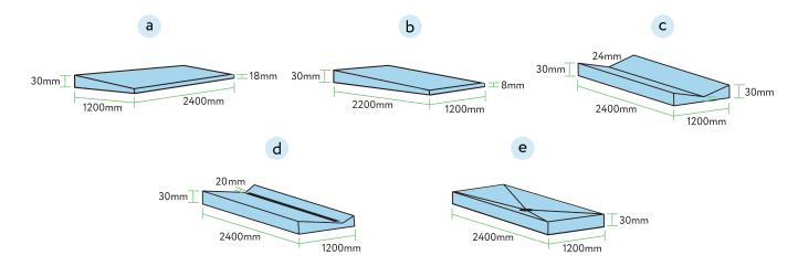
MULTIPANEL is 100% waterproof, making it an ideal screed replacement for external balconies. Utilising a combination of Long and Short Fall graded panels can help you achieve the fall to waste outlets required.
